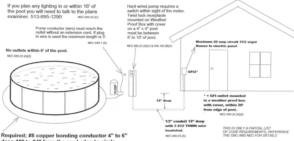
deep 18" to 24" from the pool edge to circle the entire pool and connected to the motor ground.
